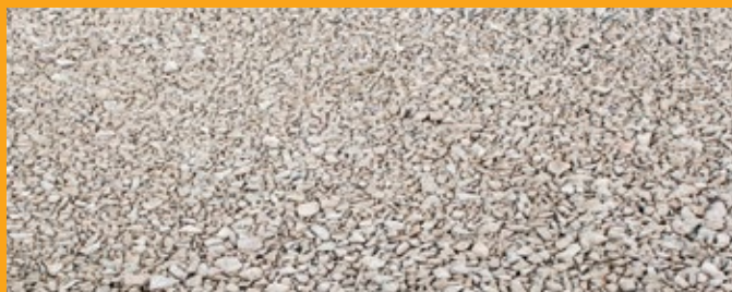
Laying course 2-6mm clean crushed stone
