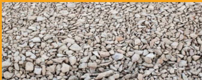
Lower sub-base layer 10-63mm clean crushed stone
